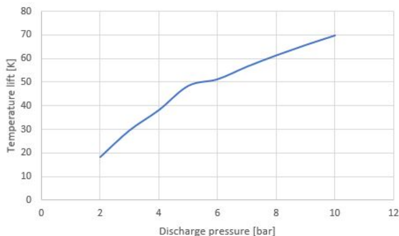
Figure 7.9: Temperature lift in the compressor for different discharge pressures. As expected the temperature increases with higher pressures and so the lift increases. For the lower discharge pressures the rise is slightly more than for higher discharge pressures.
