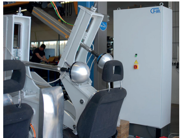
Figure 13.8.3 Strength test on seat.
