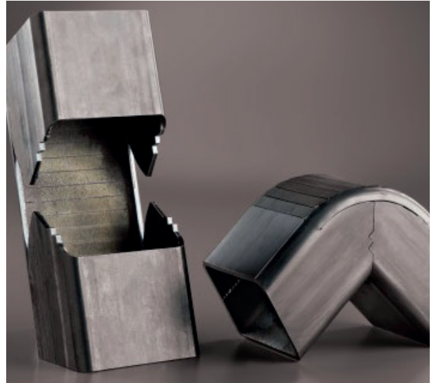
Figure 13.7.2 Tube where profile laser cutting is employed
