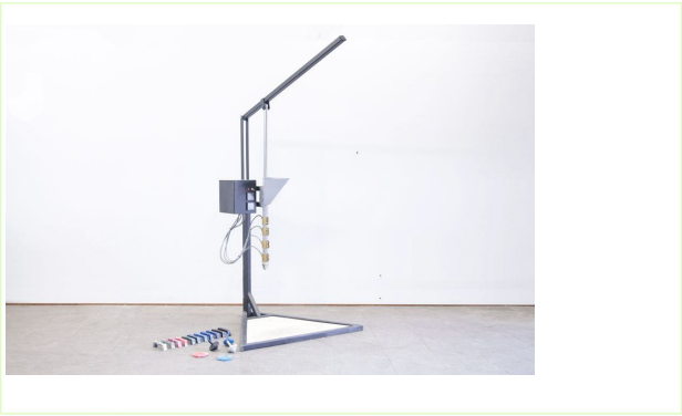
image / figure 2 Precious plastics, simple and cheap injection moulding machine
