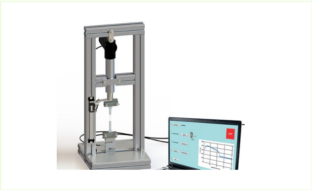
image / figure 1 Low-end tensile tester (LETT), developed by the TU Delft
