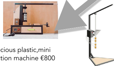
5 Precious plastic, open source injection machine €130 (self build)
