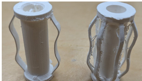
3D printed claps. Printed in different orientations and structures.
