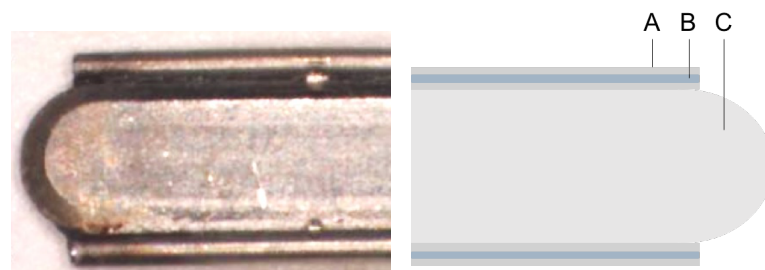
Figure 3: The tip of the electrosurgical cutting blade with both fibers attached to it. Left, a picture of the prototype [7]. Right, a schematic image of the electrosurgical blade (C) with the partly exposed fibers (B) covered in a metal sleeve (A).
