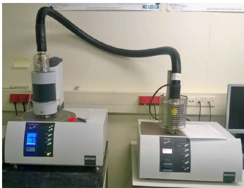
Fig. 3-9 TG-449-F3-Jupiter instrument for TGA
