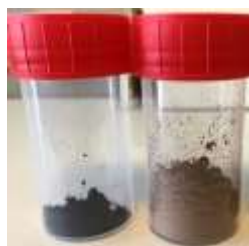
Fig. 6-6 Color change of BA sample (left-MBA, right-MTBA)
