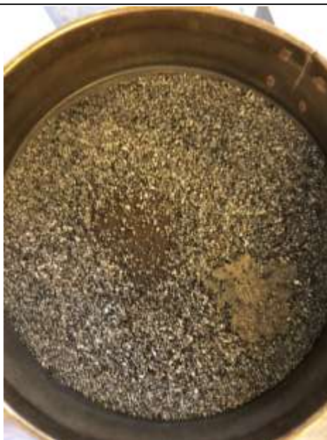
Fig. 3-2 Dry sieving test
