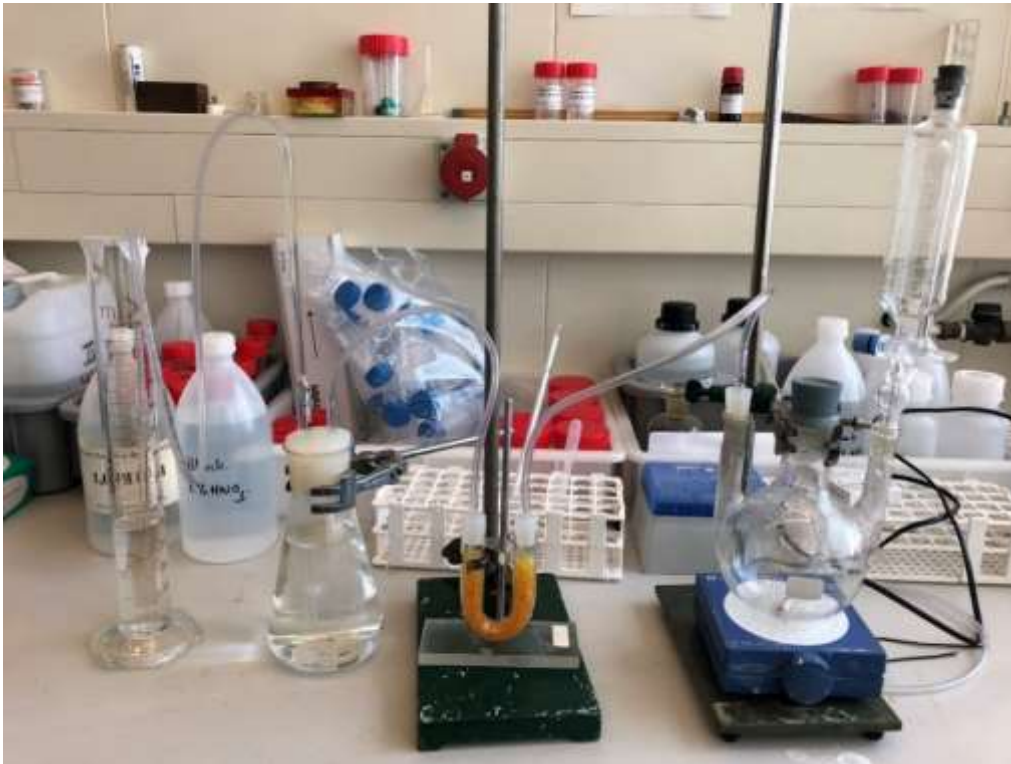
Fig. 4-7 Testing system to determine metallic aluminum content
