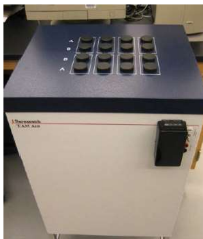
Fig. 3-8 TAM-Air-314 thermometric isothermal conduction calorimeter with 8 channels
