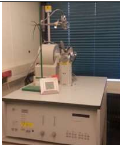
Fig. 3-5 Philips PW 1830 powder X-Ray diffractometer
