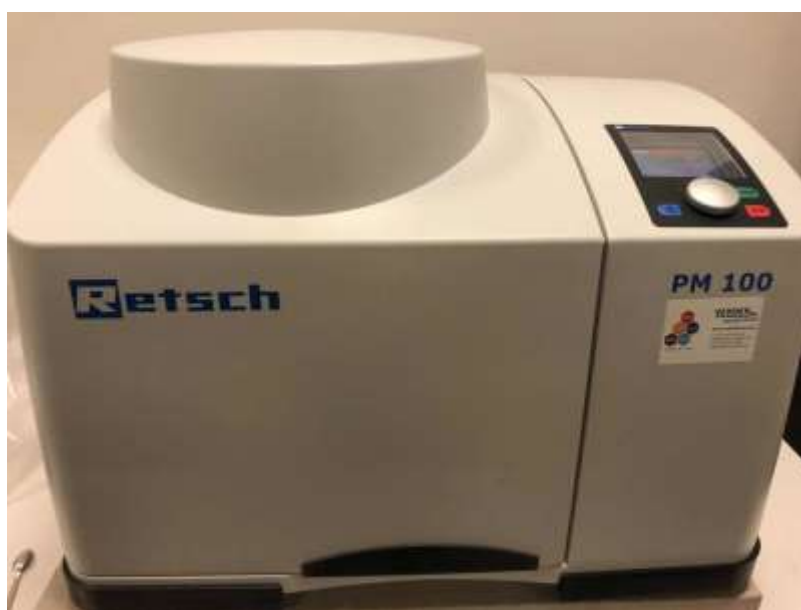
Fig. 3-7 Retsch PM100 planetary ball miller
