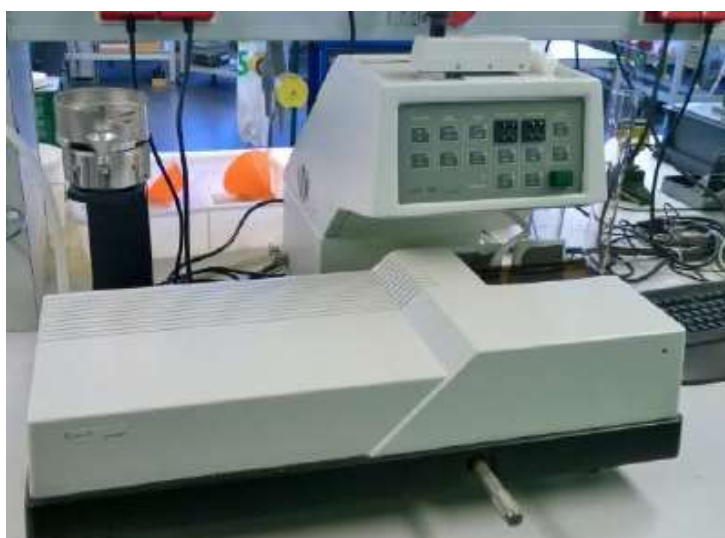
Fig. 3-3 Eye Tech laser diffraction machine
