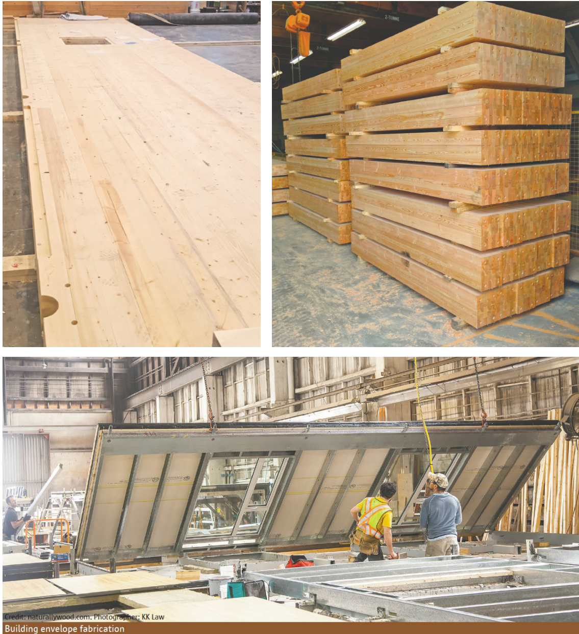
Figure 5. Prefabricated CLT floor, glulam columns, and facade elements (Canadian Wood Council, 2019)
