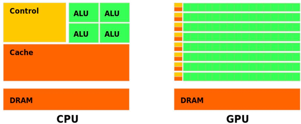
**Figure 3.** Illustration of the ratio of Control (yellow) and Cache (orange) to Arithmetic Logic Units (green) for a GPU (left) and a CPU (right) system.
