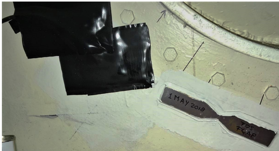
Figure 8.49: Installed sensor together with strain gauges on board of USCGC 'Bertholf'
