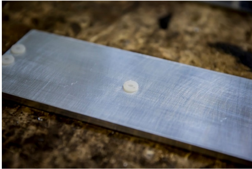
Figure A.77: Abraded surface should look dull
