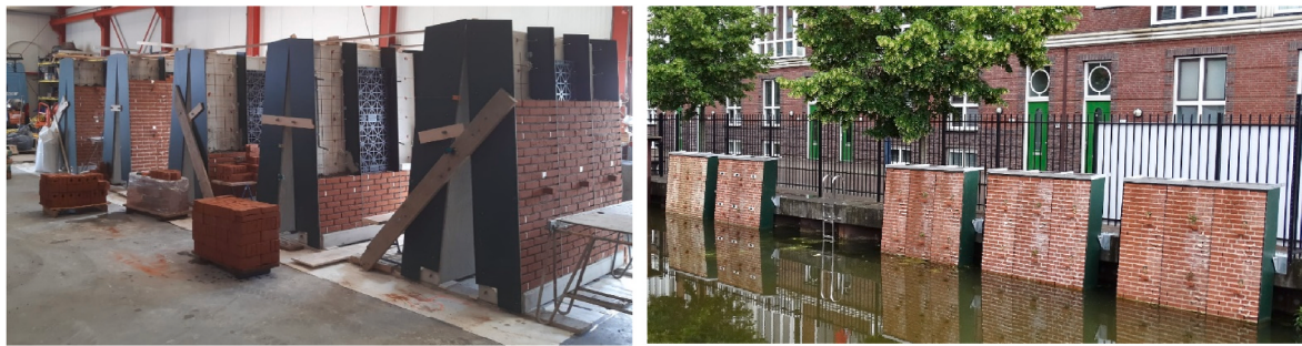
Fig. 2. left: Building of the walls; in the middle panel space between the masonry and the concrete slab is left for pouring of the substrate (the plastic containers had only a safety function); right: South facing walls placed at test location.
