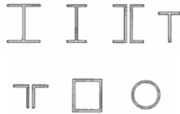
Figure 2.4.1. Typical cross sections for truss members. Edited from SteelConstruction. (n.d.).
