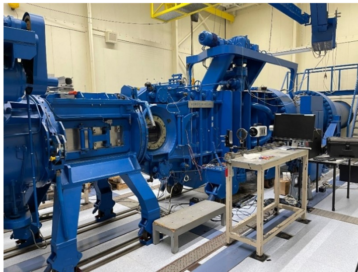
Figure 3.1: The TST 27 blowdown wind tunnel
