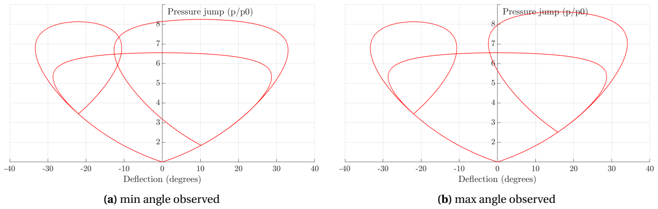
Figure 5.26: Shock polar analysis for the case with a strong interaction at a 22° shock generator
