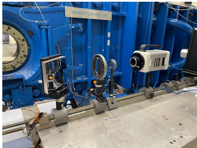
Figure 4.2: Configuration of the knife edge for the tests
