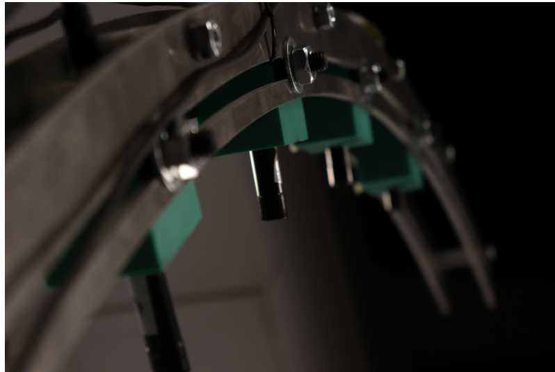
Figure 3.4: Microphones mounted on the dynamic arc for directionality measurements
