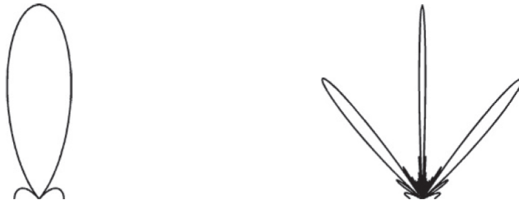
Figure 2.19: Main lobe at low frequency (and lower resolution)(left) and additional side lobes at high frequency (and better resolution)(right) [28]
