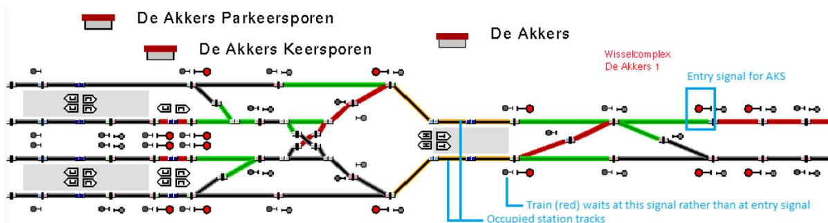
Figure 4.3: The traffic jam at *De Akkers*, caused by an entering train wanting to enter an occupied track
