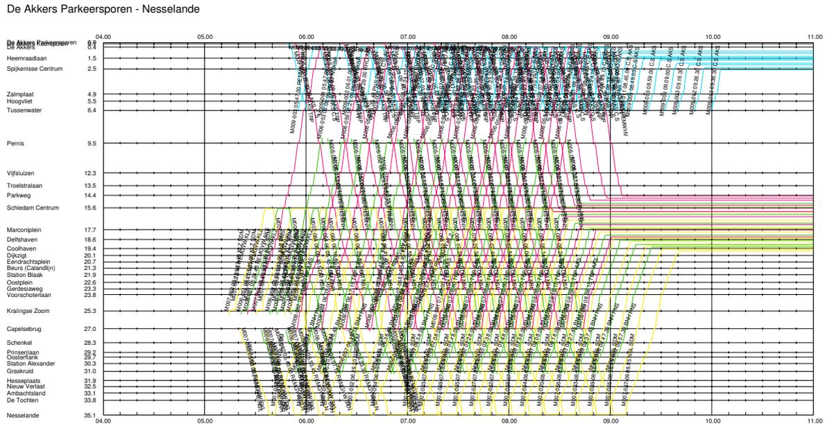
Figure 4.2: Space-time diagram demonstrating blockages at terminal station (horizontal lines represent stationary trains)
