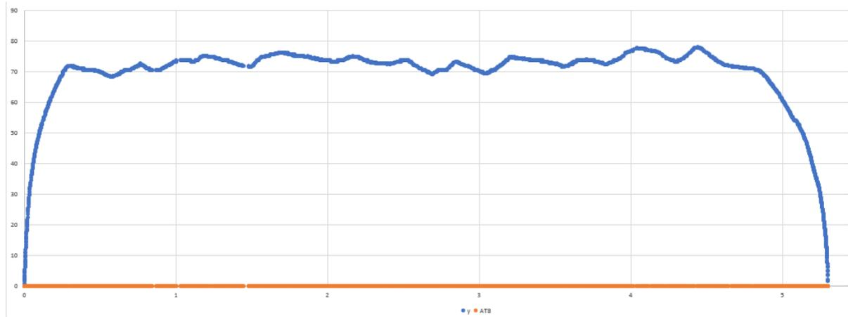
(a) Speed profile of a real train between *Rhoon* and *Slinge* (Graph courtesy of RET)
