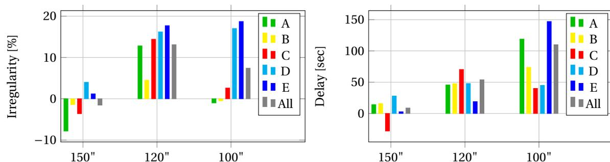
Analysis of the performances per section has revealed that a sections with regularly planned headways perform better in regularity than sections with irregularly planned headways. For the case of dis-punctuality, the number of train and therefore the length of the headway is important. Sections with fewer services are more punctual than sections with more services.
