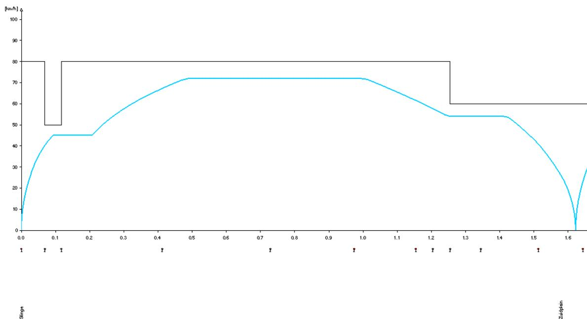
(b) Speed profile of a simulated train between *Slinge* and *Zuidplein* (Graph courtesy of RET)
