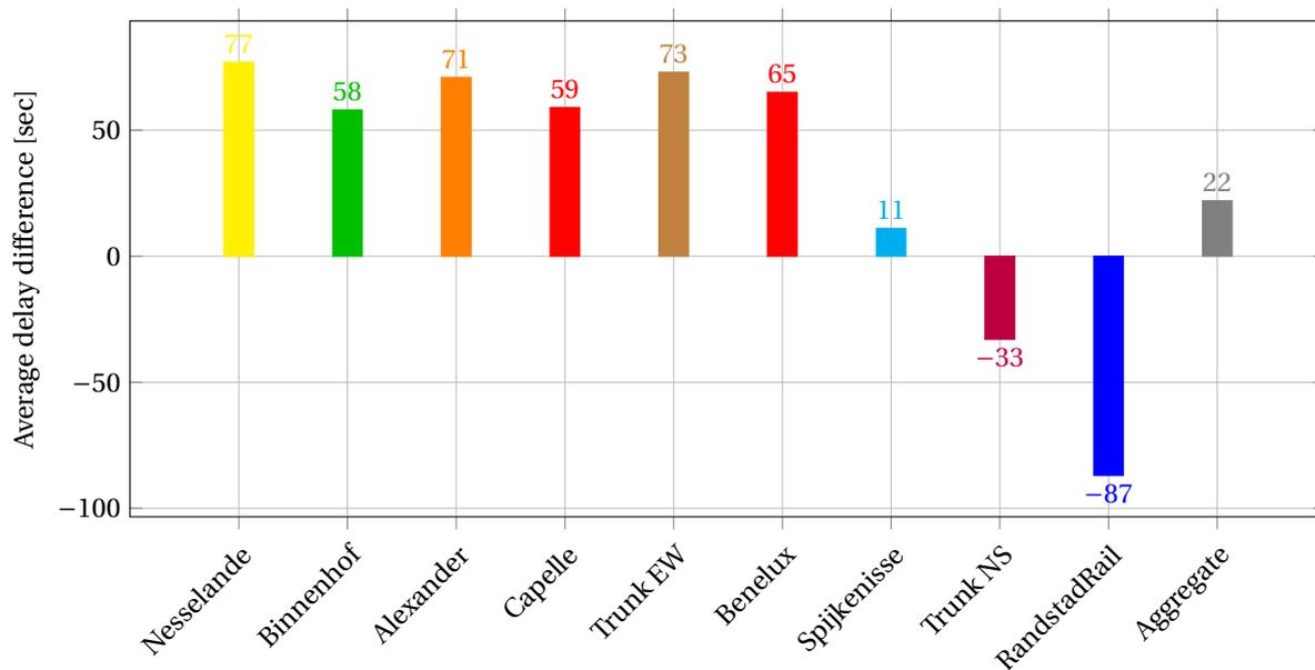
Figure 4.21: Difference (in seconds) per section in terms of average delay of performance of simulations compared with real data
