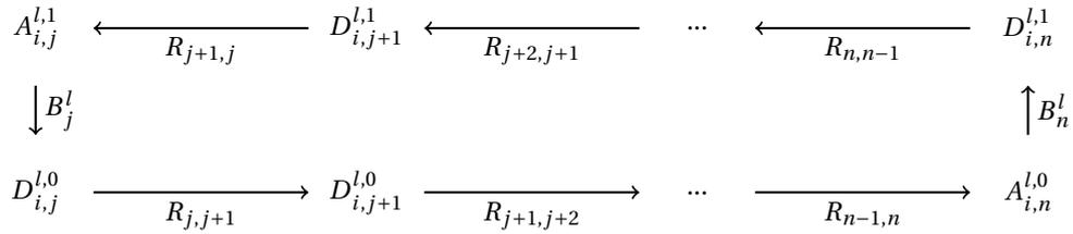
Figure 5.1: Graphical representation of departure times, arrival times, running times and reversing times along line  $l$
