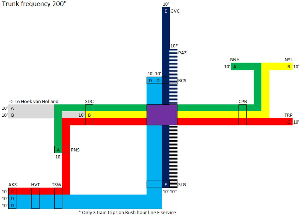
Figure 4.16: Schematic overview of the lines and frequencies operated in the current timetable
