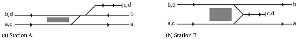
Figure 3.2: Two different layouts for a station where trains can be reversed, from Landex and Jensen (2013)
