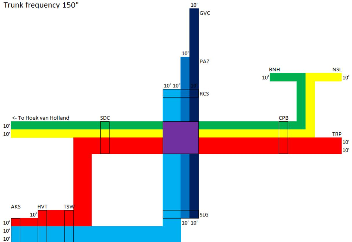
Figure 5.5: Schematic overview of lines and frequencies operated in Scenario 150
