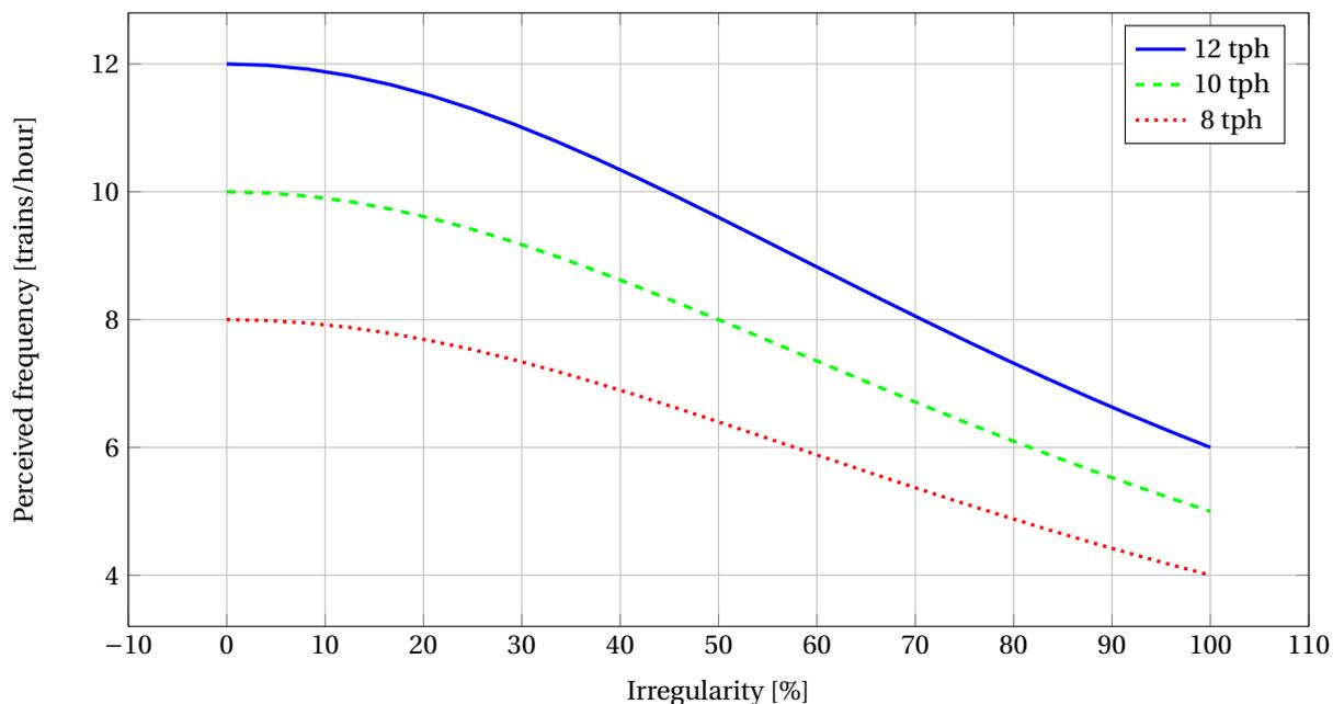
Figure 2.2: The relationship between irregularity and perceived frequency (adapted from Van Oort and Van Nes (2009b))
