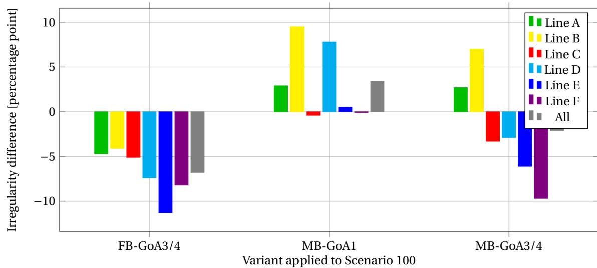
Figure 6.7: Difference in irregularity between upgrade variants and current variant *FB-GoA1* for Scenario 100
