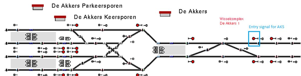
(b) Signalling situation of *De Akkers* after some signals are removed
