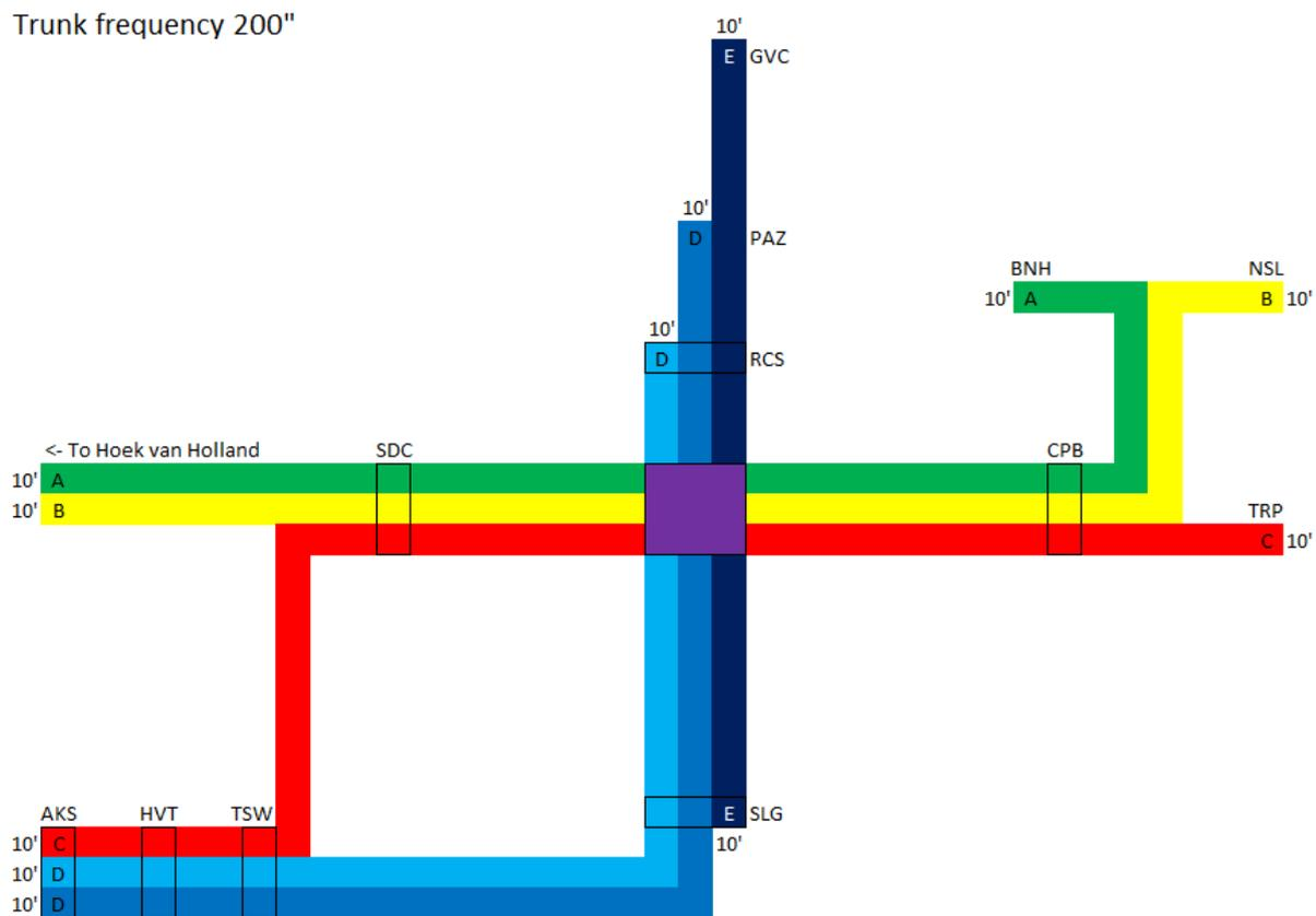
Figure 5.3: Schematic overview of lines and frequencies operated in the base scenario
