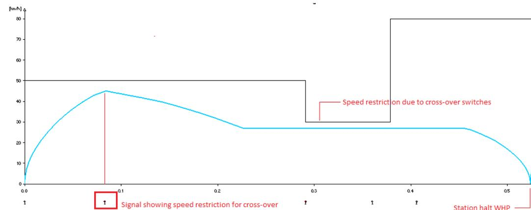
(b) Speed profile of a simulated train between *Rijnhaven* and *Wilhelminaplein* using switch-over points (Graph courtesy of RET)
