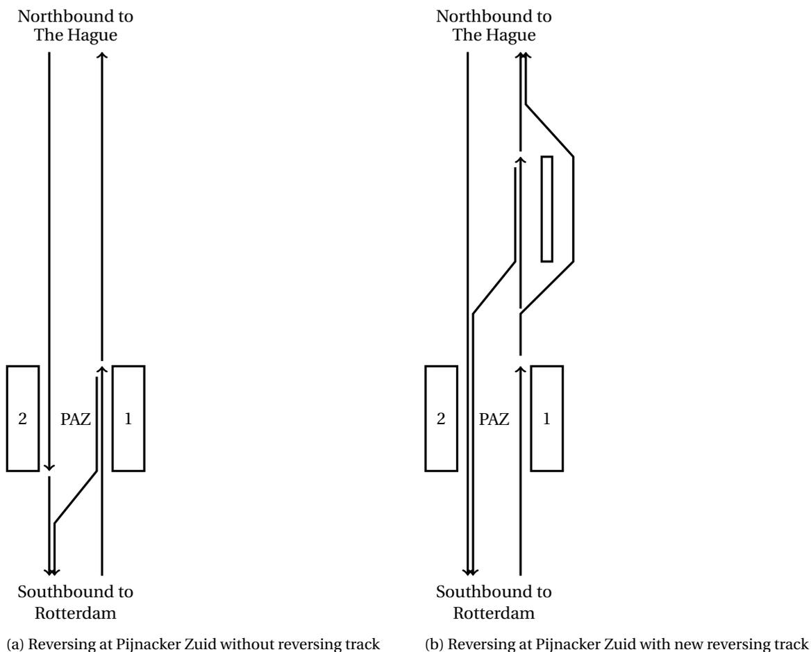
Figure 5.4: Schematic layout of Pijnacker Zuid before and after construction of the reversing track
