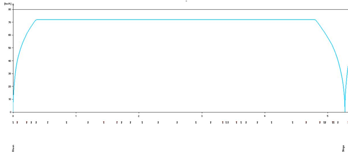
(b) Speed profile of a simulated train between *Rhoon* and *Slinge* (Graph courtesy of RET)
