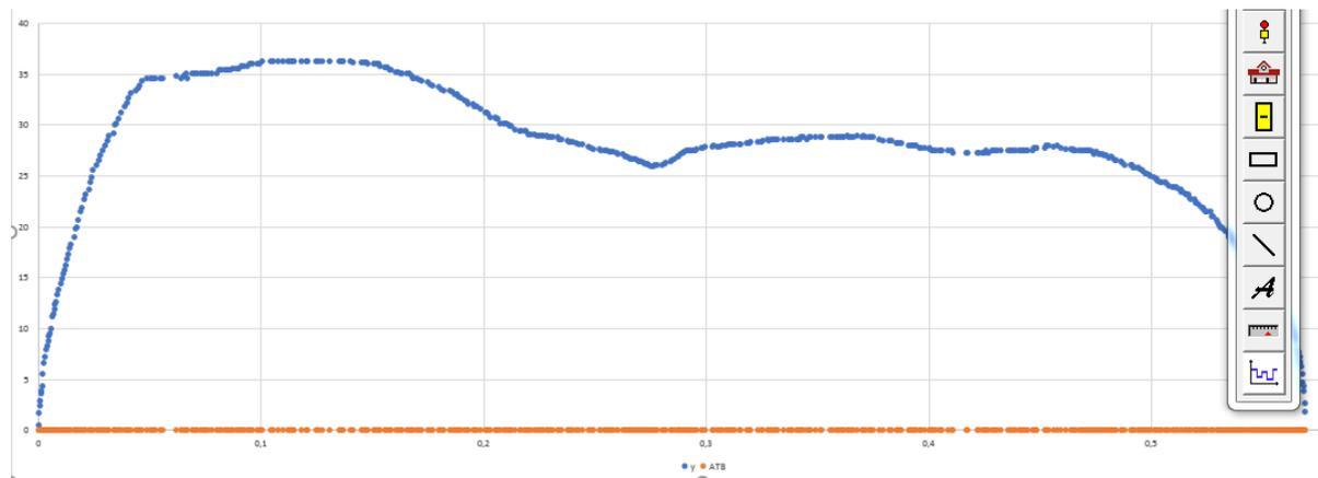
(a) Speed profile of a real train between *Rijnhaven* and *Wilhelminaplein*, using switch-over points (Graph courtesy of RET)
