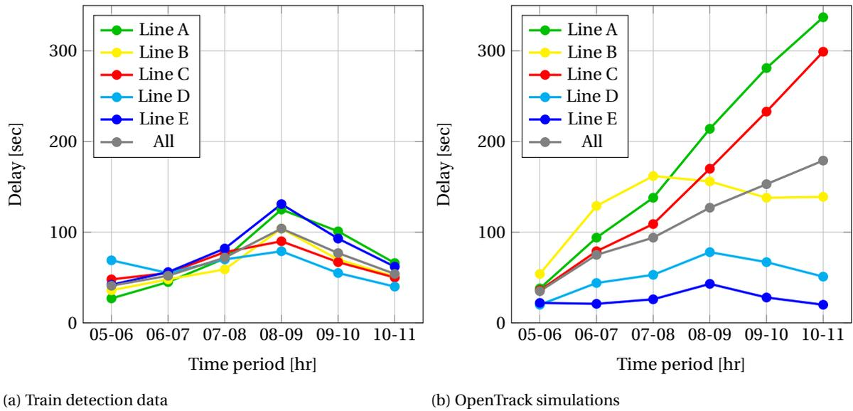
Figure 4.22: Overview of average delay per line per time period, for the real train detection data and OpenTrack simulations
