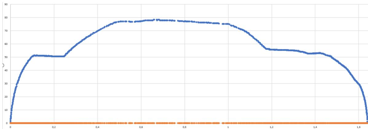
(a) Speed profile of a real train between *Slinge* and *Zuidplein* (Graph courtesy of RET)
