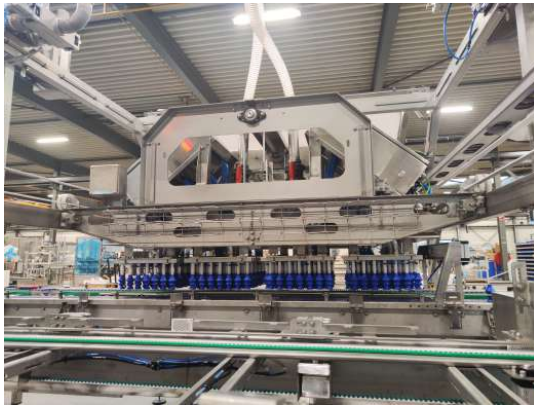
(a) The space that can be seen between the sets of suction cups can be adjusted, if required by the configuration.
