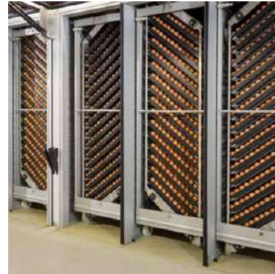
Figure 1.3: An example of a setter incubation cell with tilted setter trays on trolleys [5]
