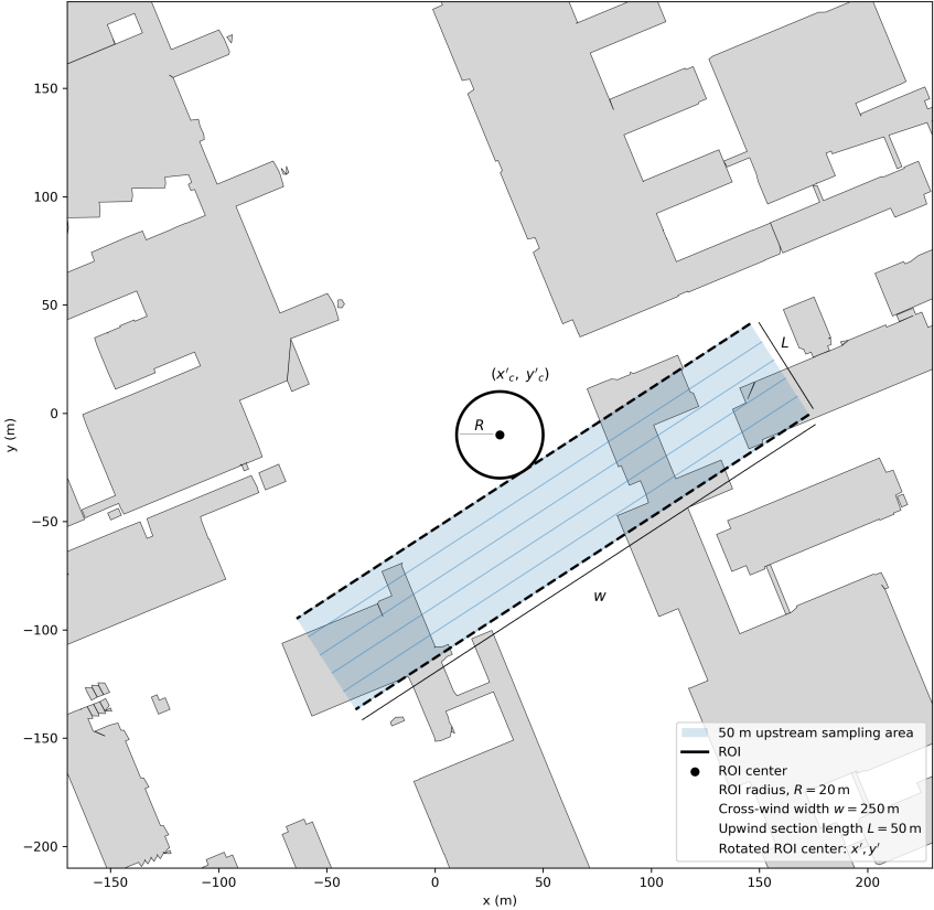
Figure 3.14: Visualization of the planar blockage-ratio in the reference layout. The figure shows the region of interest (ROI), the entry location x'_{entry} , the cross-wind corridor of width w , and the upstream section of length L used to compute the mean planar blockage ratio. The geometric quantities are defined in the rotated wind-aligned coordinate system (x', y') .
