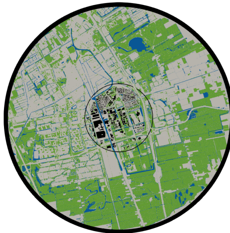
Figure 3.7: Top view of the computational domain. Buildings are modeled only within the inner circle (study area). The outer region contains no buildings and it is modeled as flat surface with different layers (terrain, vegetation and water). The different colours indicate: buildings (dark grey), vegetation (green), water bodies (blue), and terrain (light grey).
