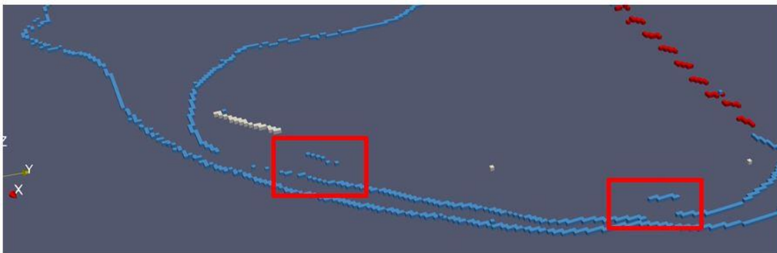
Figure 18: Classified furniture objects (white), stair seed voxels (red) and horizontal seed voxels (blue). The furniture elements in the red box cannot be detected as furniture objects.
