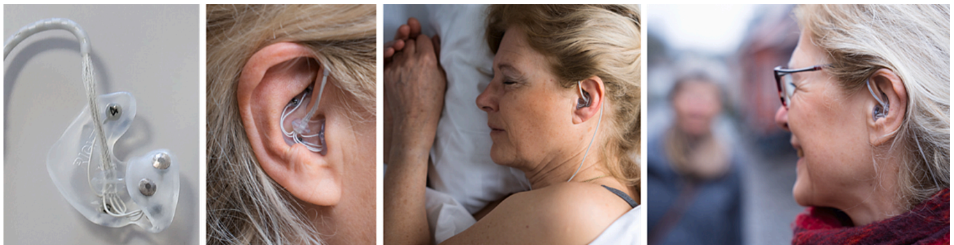
Fig. 1. Example of ear-EEG. Left to Right: Individualized earpiece with dry-contact electrodes. Ear-EEG ear-piece in the ear. Ear-EEG used for sleep monitoring. Ear-EEG used in real-life monitoring. Photo: Center for Ear-EEG, Aarhus University. Image used with permission from Center for Ear-EEG, Aarhus University. The person depicted provided informed consent.
