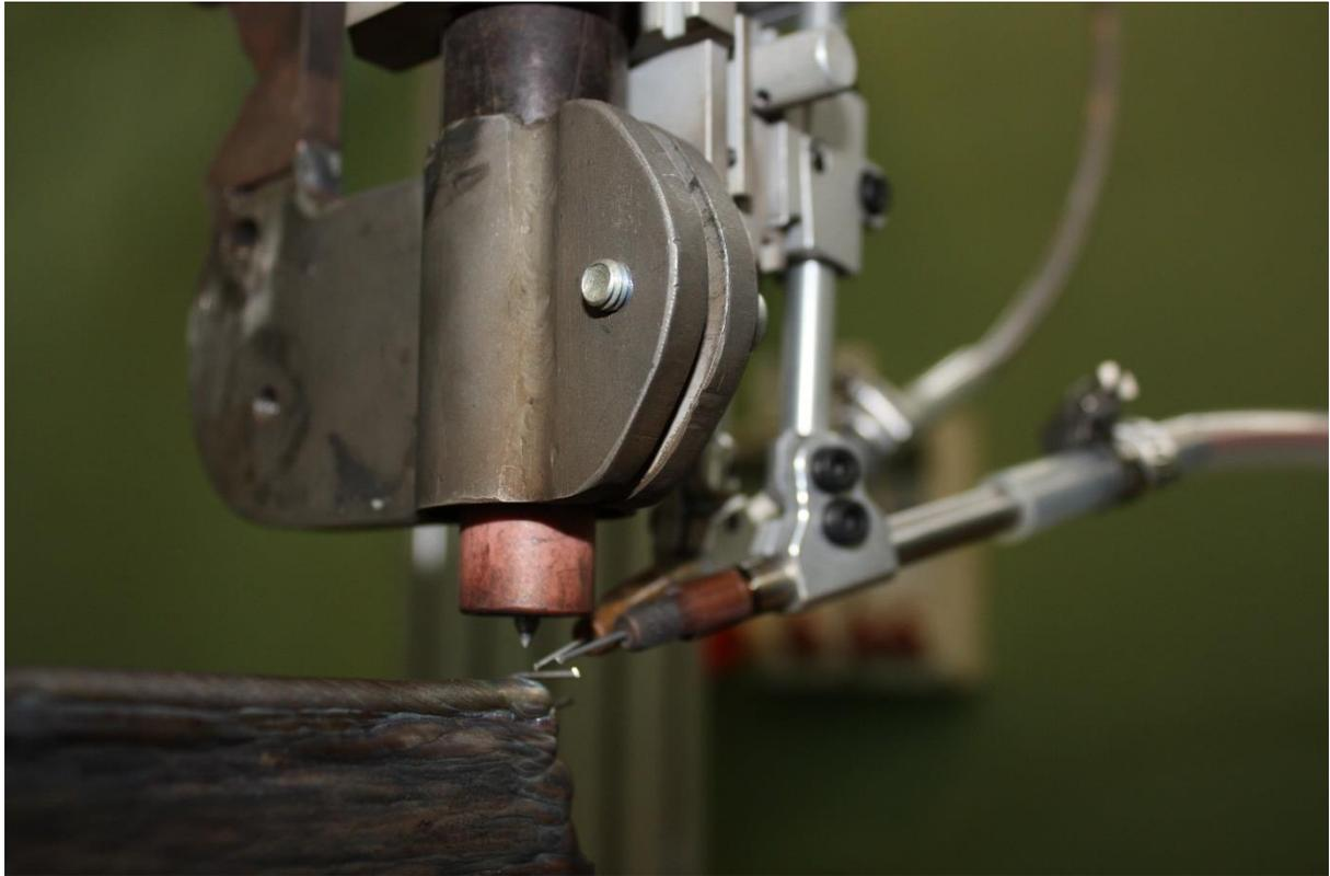
Figure 20: Photograph of welding torch with two wire feed holders was moved over a clamped and stationary workpiece for simultaneous wire feed at the electrode
