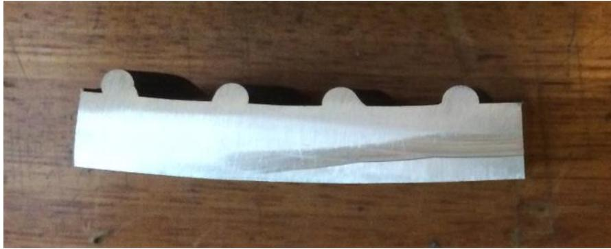
Figure 29: Warping of the substrate due to welding on the face of the plate
