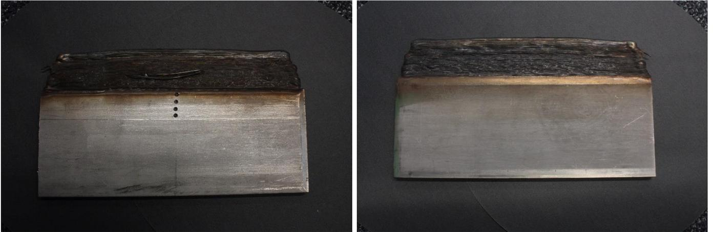
Figure 40: Welded AISI 316L/AISI 430L graded structure
