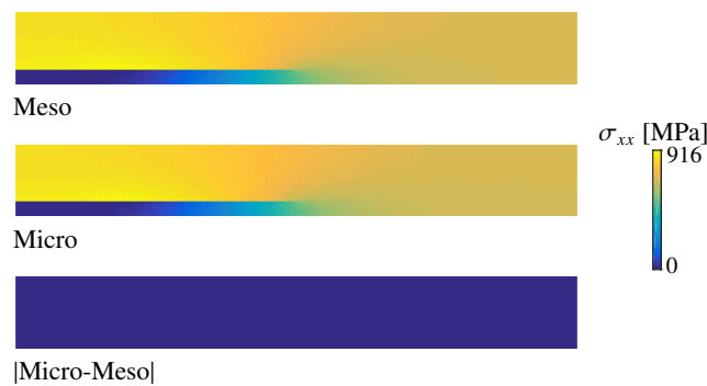
Figure 3. Comparison between \sigma_{xx} field from mesolevel analysis of TCT test and reconstructed \sigma_{xx} field from micromechanical analyses with the same averaged strain histories.
