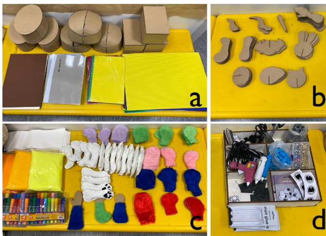
Fig. 3. Examples of the construction toolkit and materials at our co-design workshop for building up a robot prototype: (a) varied shapes of torsos [top], varied hard materials [bottom]; (b) varied shapes of heads, legs, and arms; (c) varied soft materials; and (d) mock-up interactive attachments, e.g., cameras, speakers, interaction sensor.
