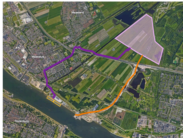
Figure 5.5: Map showing truck route from groyne cells to placement polder (purple) and Pipeline from anchorage to placement polder (orange)
