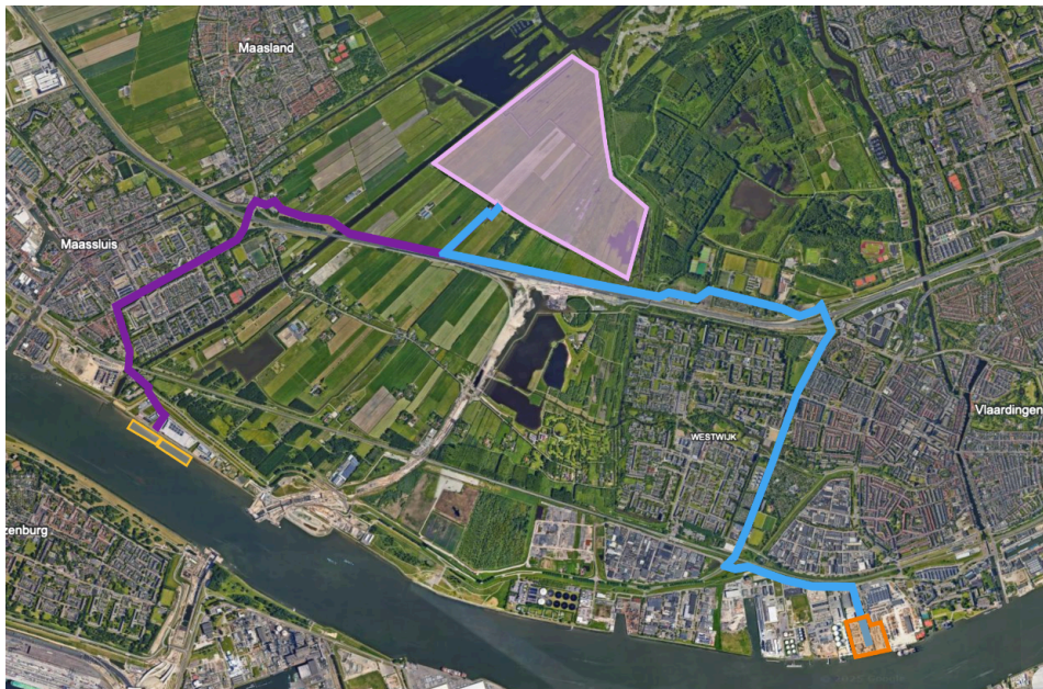
Figure 5.7: Map showing the route for the sediment over land, purple indicates the route from onshoring to drying location, and light blue the route from drying to concrete manufacturer.
