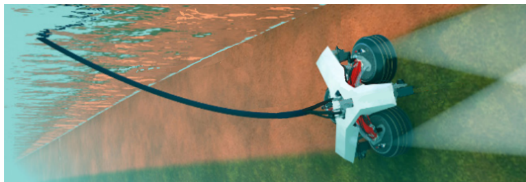
Figure 1-1: Render of the Fleet Cleaner robot cleaning the side of a ship hull while underwater.
