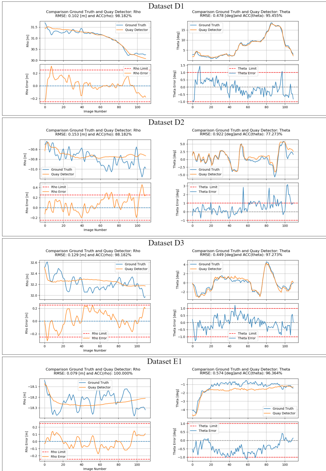
Figure 5-9: Comparison between ground truth and EKF-filtered quay wall tracker estimation of \rho and \theta . In comparison with the unfiltered measurements shown in Figure 4-13, one particularly interesting observation can be made: the \rho measurements are clearly less noisy, so much that the ground truth measurements are the ones appearing to be noisy.
