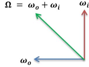
Figure 3. Total angular velocity vector.
