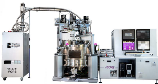
Fig 4: Prototype Cryogenic Wafer Prober. The tool allows full 300mm e-test automation at a wafer temperature of T= 1.9K.
