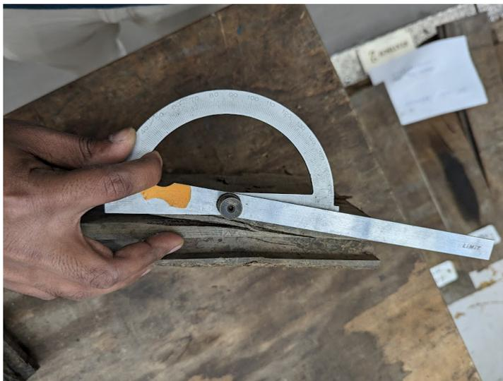
Figure 3.28: Fibre deviation angle measured on a bending tested board
