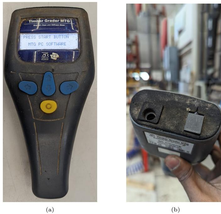
Figure 3.10: Timber grader MTG equipment
