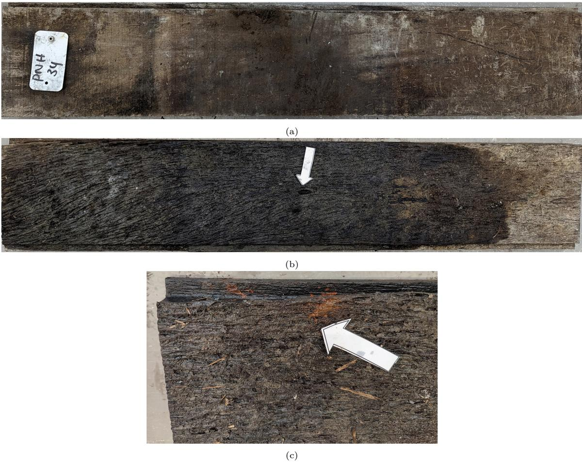
Figure A.4: PNH34 (a) Side W (b) Side E (c) Part of groove in side E decayed and chipped off
