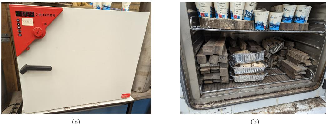
Figure 3.29: Moisture testing oven maintained at a temperature of  $103^{\circ}$
