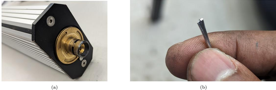
Figure 3.15: (a) Drilling head (b) Drill needle
