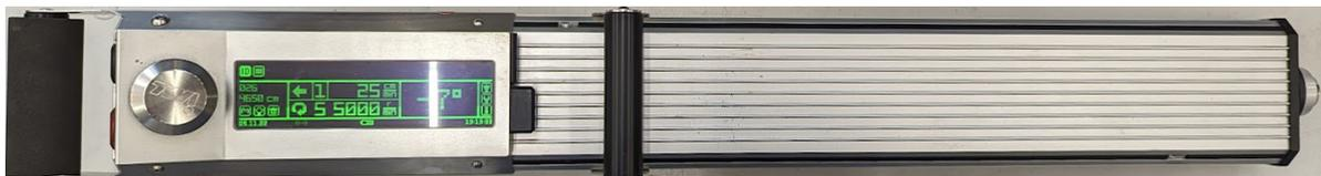
Figure 3.14: IML RESI PD-400 RPD testing equipment
