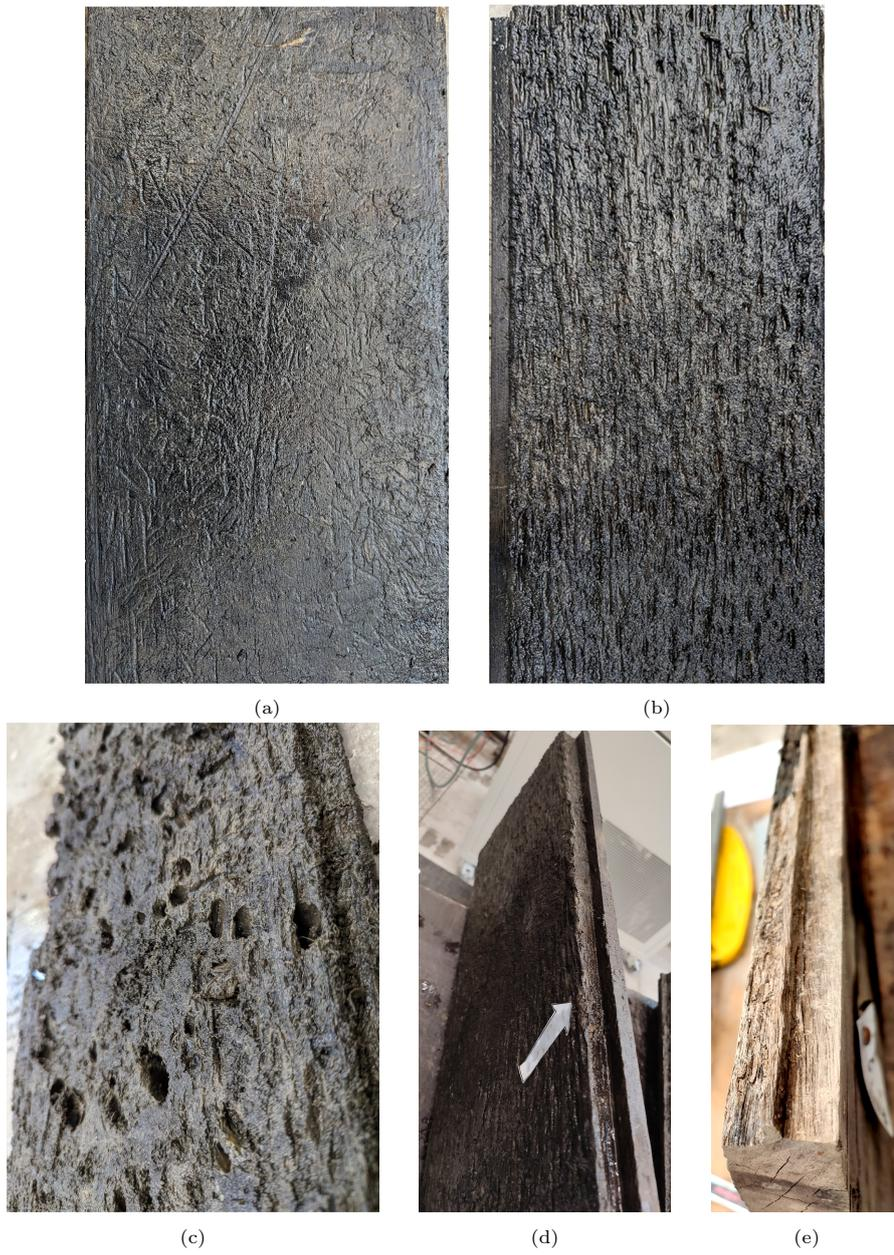
Figure 3.7: Types of decay at different locations on each board (a) W side (b) E side: striped decay (c)E side: decay holes (d) E side: thickness wise decay of the groove (e) E side: thickness wise decay of the tongue
