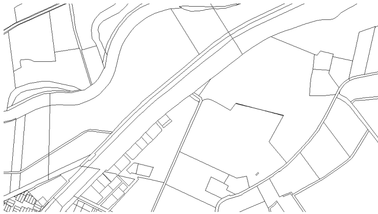
Figure 2.4: A 2D cadastral map : points, lines and polygons are used to model parcels in 2D space
