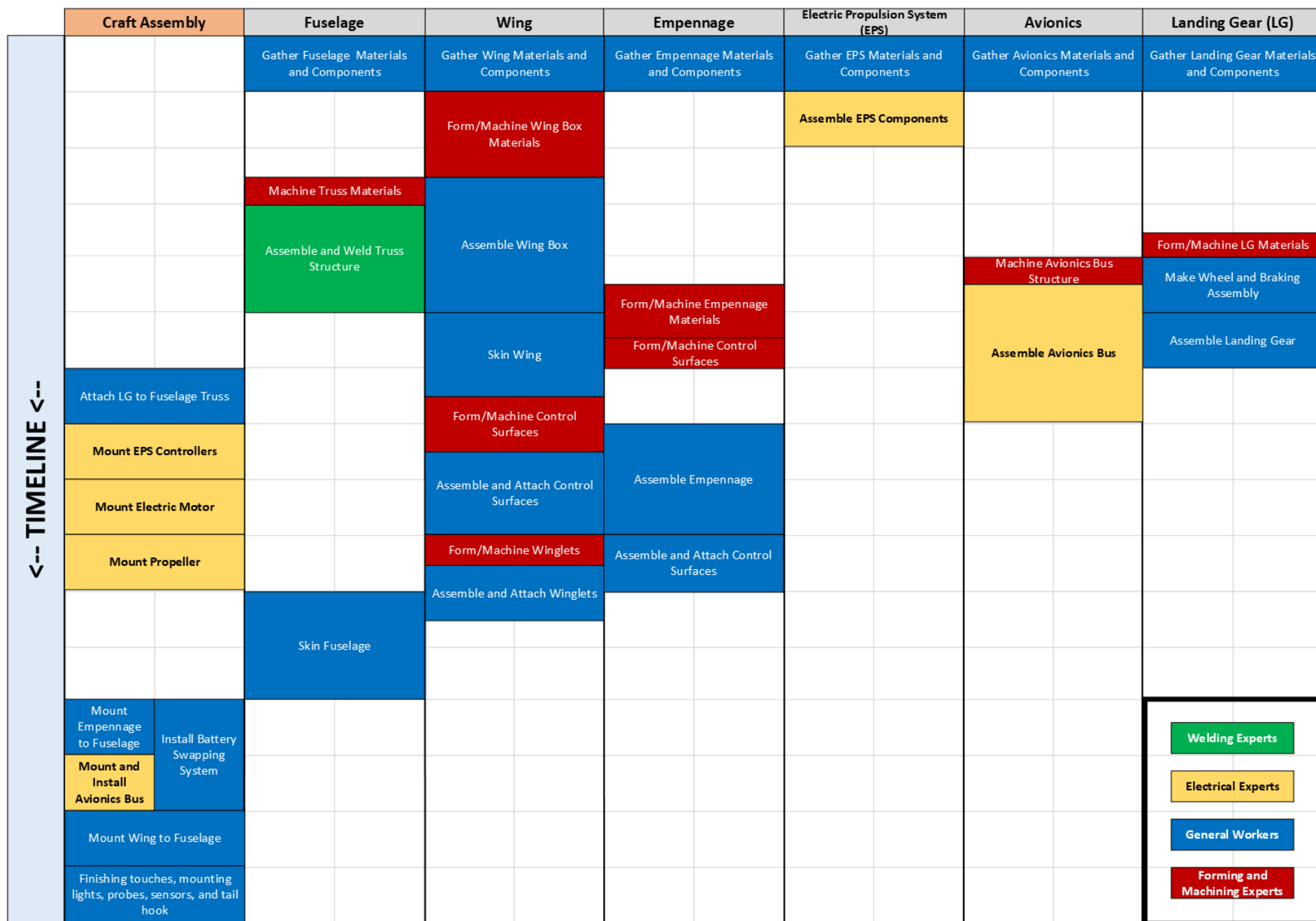
Figure 11.7: Manufacturing plan of MARCUS-T .
