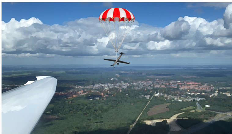
Figure 8.17: MARCUS-T with a deployed parachute as seen from a glider.
