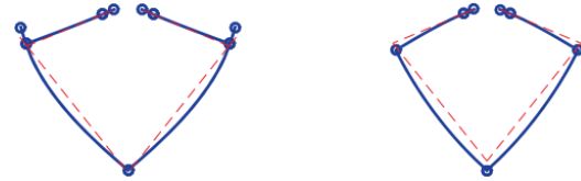
Figure 2: An attempt to dynamically balance a distributed compliant mechanism (robot arm) by rigid body balancing principles [2]
