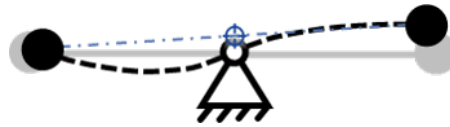
Figure 1.5: Unbalanced compliant variant of an otherwise theoretical balanced rigid mechanism after some rotation, blue indicates the translated common CoM
