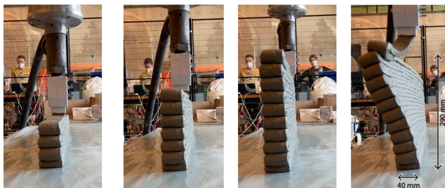
Fig. 16. Buildability test Mix C, failure after 23 layers.
