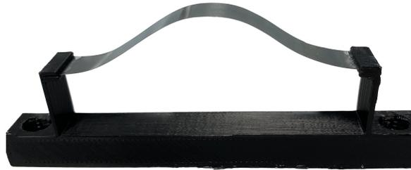
**Figure 5.10:** Prototype of metal beam with PLA supports.
