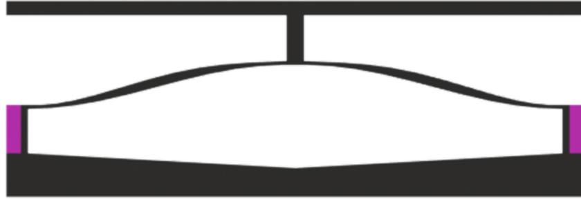
**Figure 5.6:** Design of bi-stable beam with varying thickness to create hinge-like properties
