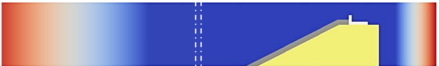
Figure 42. Relaxation zones in the model's computational domain (due to length middle part is cropped out). Post processing with Paraview.
