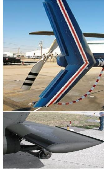
**Figure 2.2:** Gurney flap on the tail section of a Bell 222U(top),Apache(bottom) Helicopter, [11]
