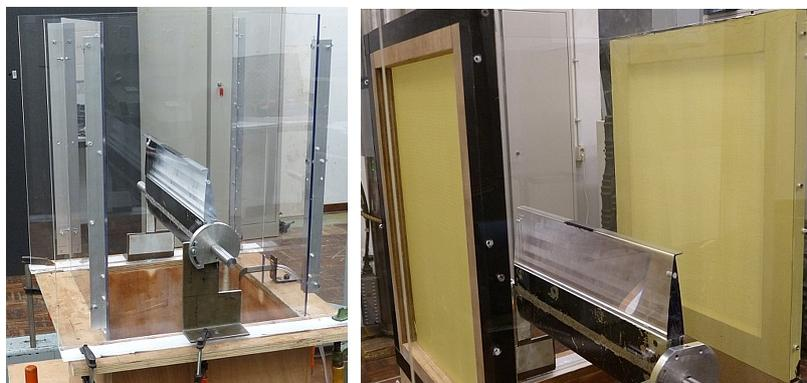
**Figure 4.3:** Test Section for PIV (left), Acoustics (right)
