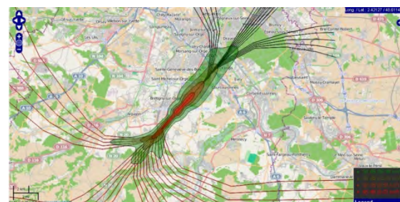
Figure 6: Noise contours associated to different trajectories, STAPES.
