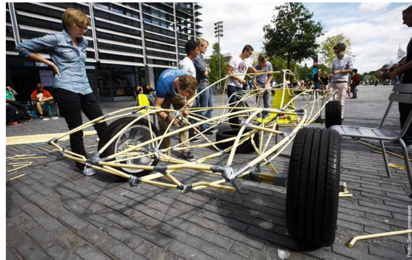
Students of the minor automotive design (faculty of Industrial Design Engineering) work on cars made of pvc pipes, tie wraps and duct tape. The minor aims to develop skills like design drawing, clay modeling and prototyping.
