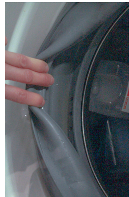
Figure 4.11 Degraded inner seal of used washing machine
