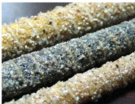
Figure 2.7: Sand-coated FRP reinforcement bars [Nilforoush and Esfahani, 2012]
