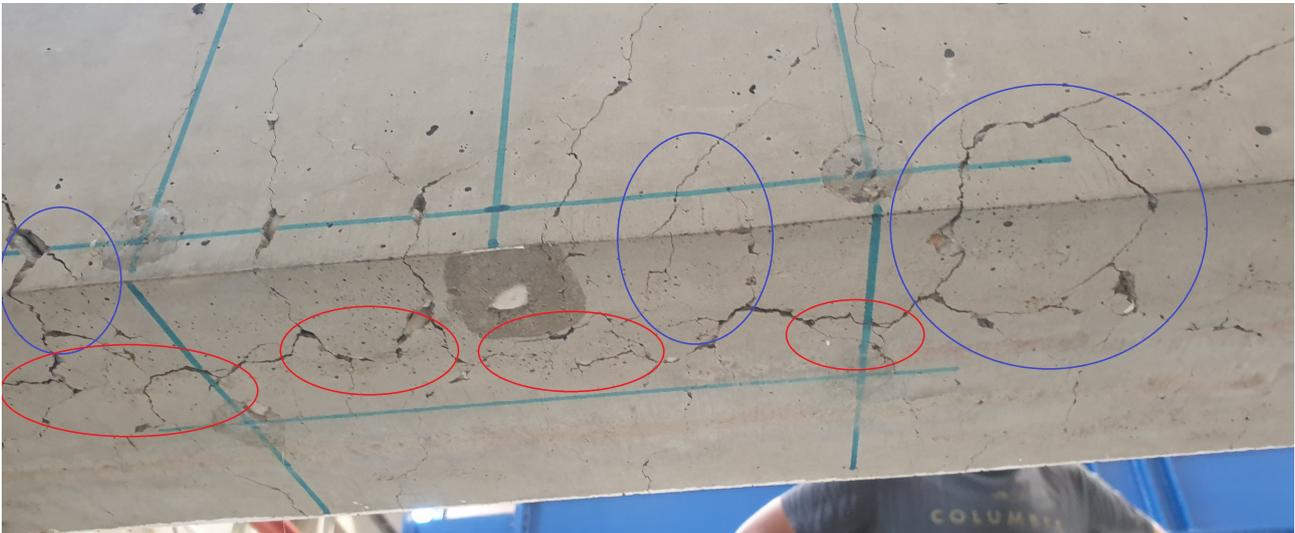
Figure 4.17: Tensile splitting cracks bottom side B-3r8-c11
