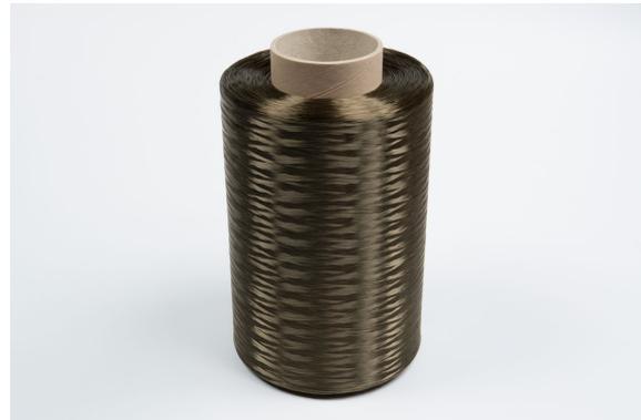
(b) Roving containing basalt fibres
