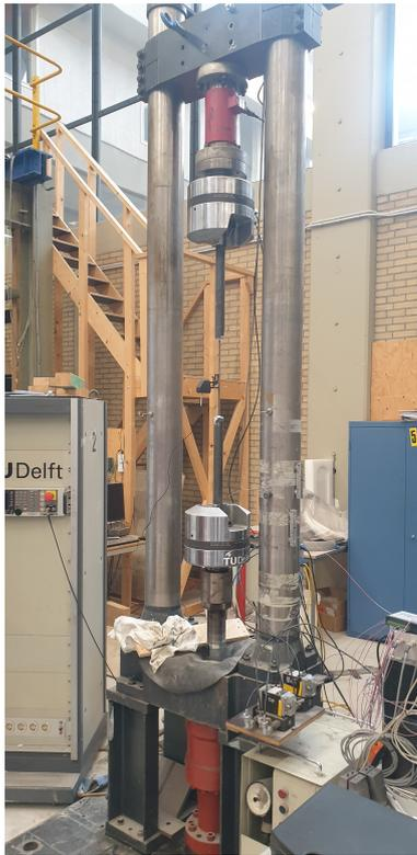
(a) Specimen loaded in direct tension testing machine
