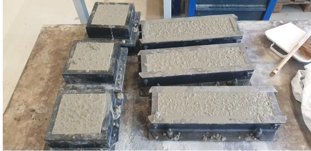
Figure 3.15: Cubes and prisms cast from concrete batch
