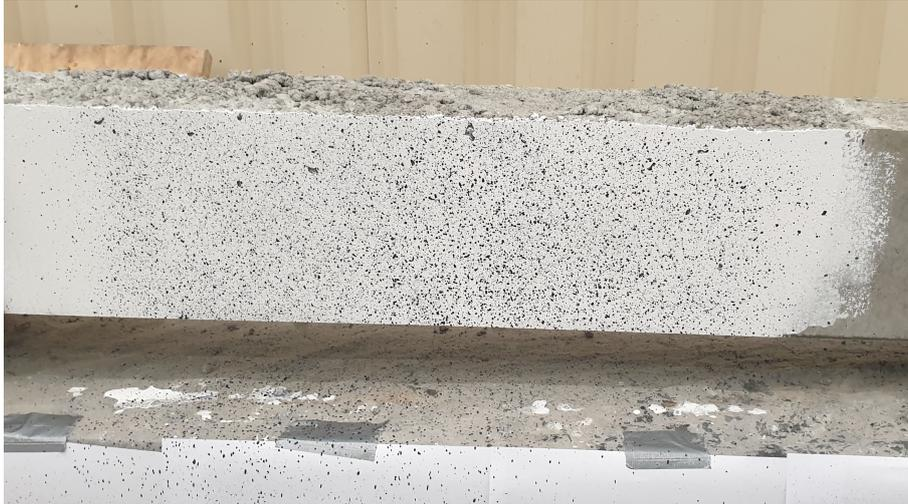
Figure 3.19: Stochastic pattern applied to beam S-3r8-c31 during test preparation
