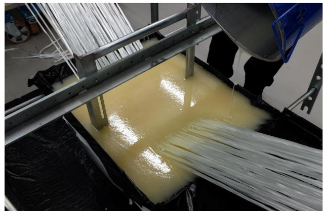
(b) Typical open polymeric resin bath
