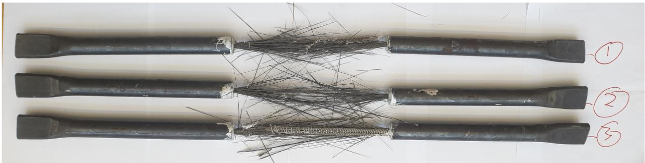
Figure 4.1: Test specimens after failure direct tension tests
