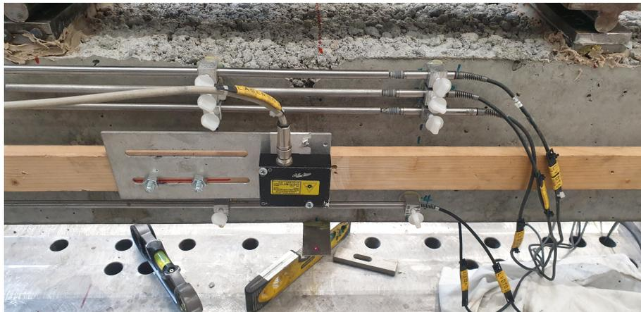
Figure 3.23: Laser device mounted to a beam specimen
