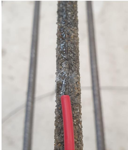
Figure 3.21: Optical fibres glued to reinforcement bar
