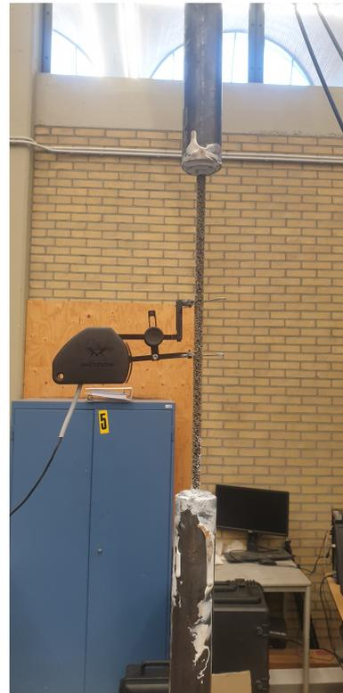
(b) Extensometer applied to the exposed part of the specimen
