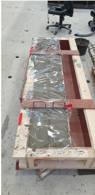
Figure 3.14: Freshly casted beams specimens 1&2 sealed with plastic layer
