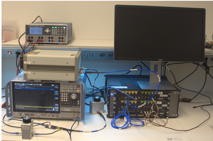
Figure 4.5: Commercial instrument validation platform for a Class-AB RF PA.
