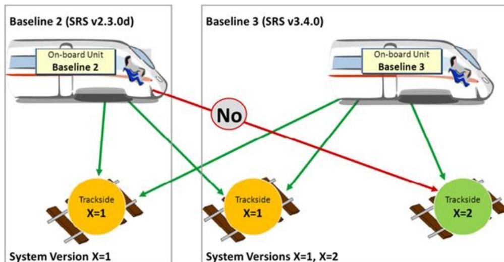
Figure 5: Compatibility between on-board compliant with a specific baseline and trackside operating with specific system version (UNISIG, 2014).
