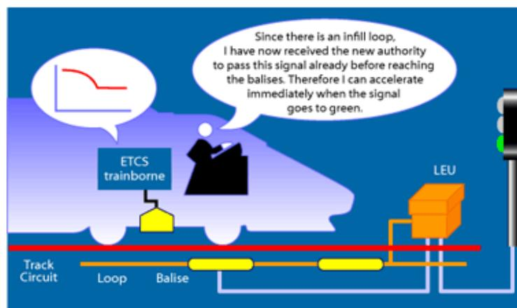
Figure 28: ERTMS/ECTS application level 1 with infill (ERTMS, 2020)
