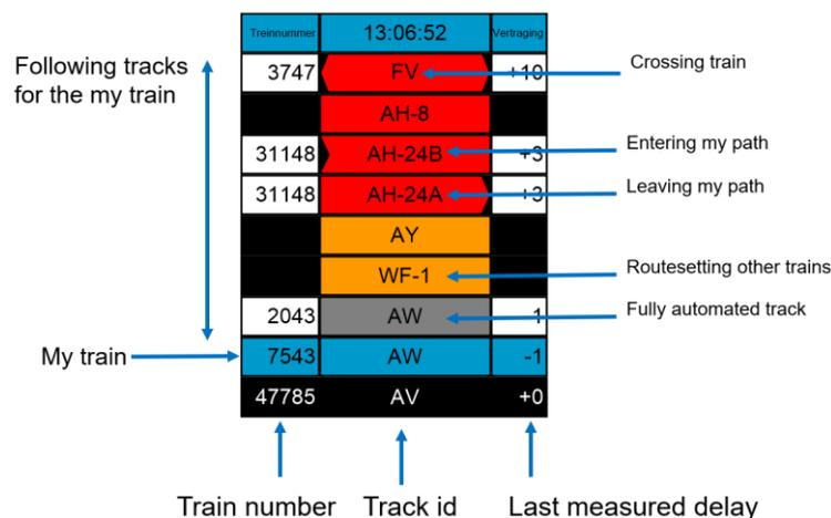
Figure 21: GUI (Graphical User Interface) by ProRail of RouteLint. Edited figure from van Luijpen (2019).
