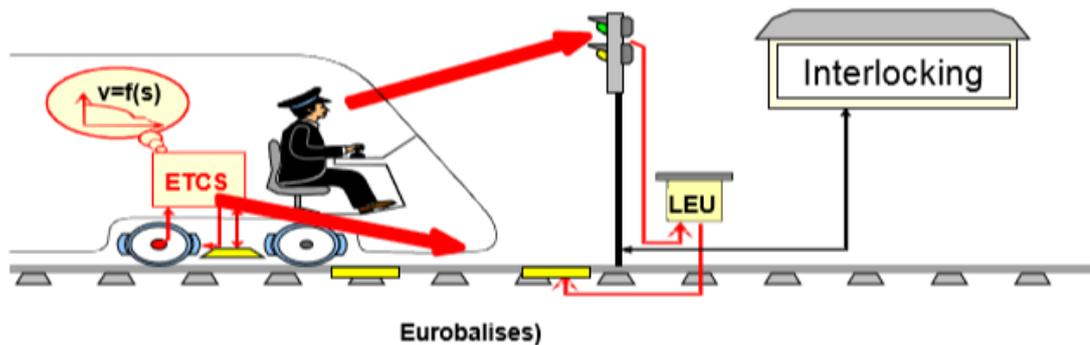
Figure 31: ETCS L1 with Limited Supervision (Stamm, 2012)
