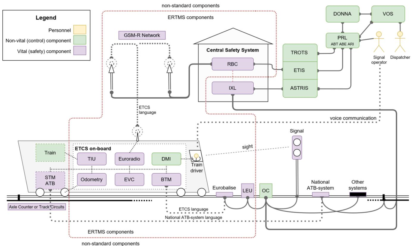
Figure 7: Sketch of used components in the planned Dutch ERTMS implementation
