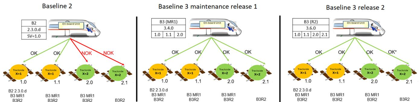
Figure 6: compatibility between SVs of on-board and trackside equipment. Edited image from Arenas (2015).
