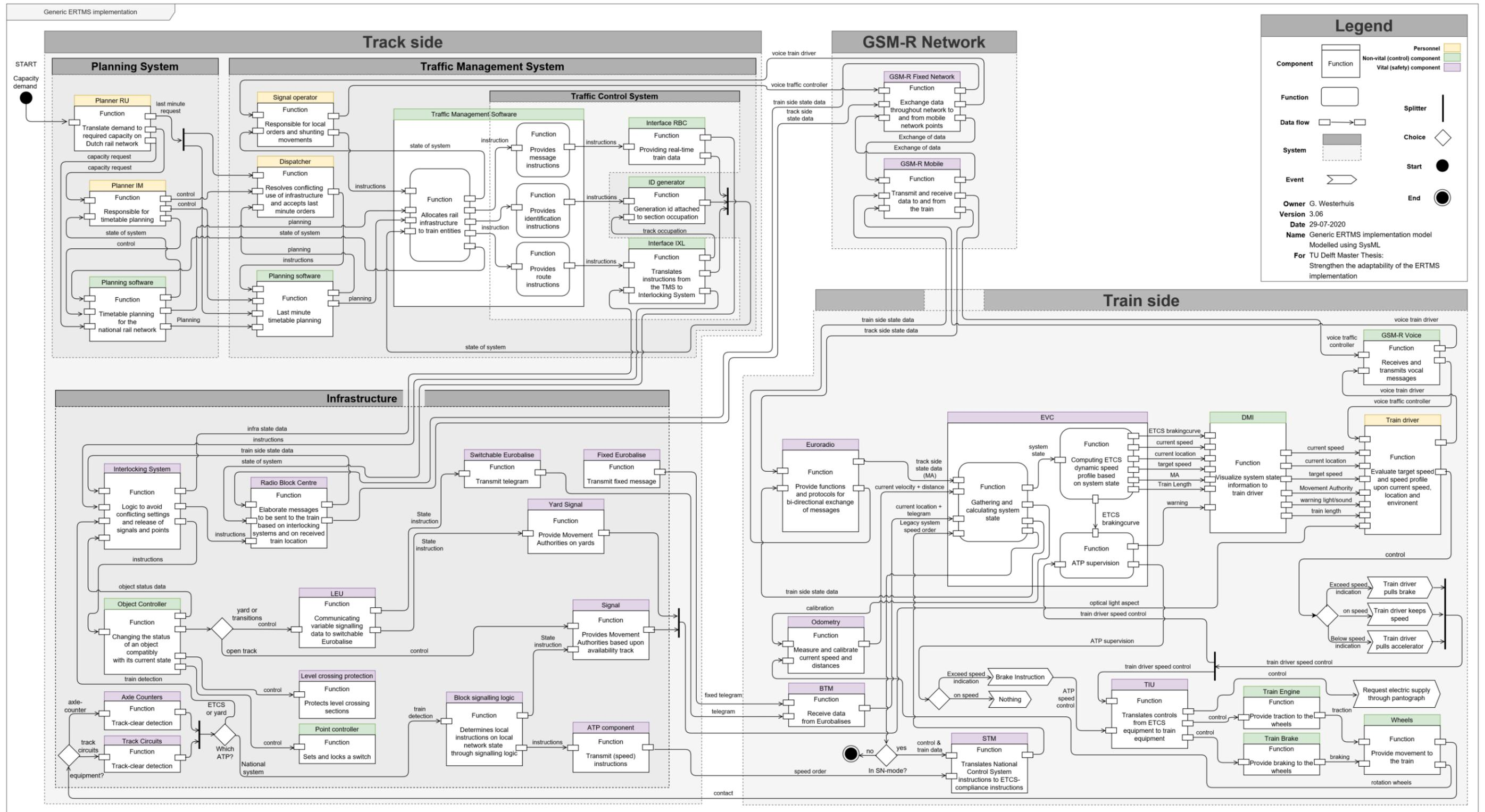
Figure 10: A generic implementation of ERTMS visualized using System Modelling Language.
