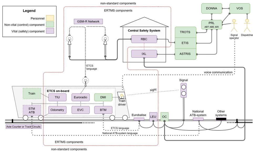
Fig. 1. Sketch of used components in the planned Dutch ERTMS implementation
