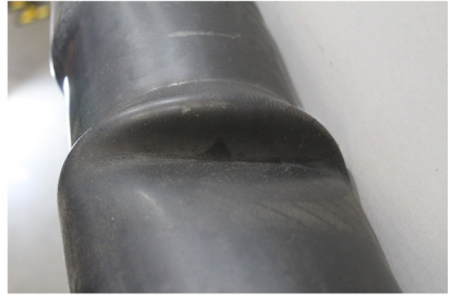
Fig. 3. – Representative plastic hinge failure mechanisms for each group of specimens linked by the same nominal wall thickness.
