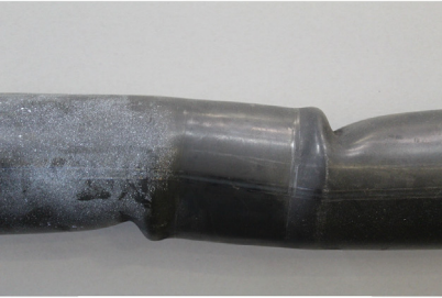
Fig. 3. – Representative plastic hinge failure mechanisms for each group of specimens linked by the same nominal wall thickness.
