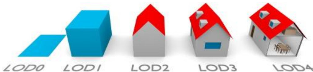
Figure 1: The five levels of detail of CityGML 2.0 (taken from Biljecki et al, 2016)
