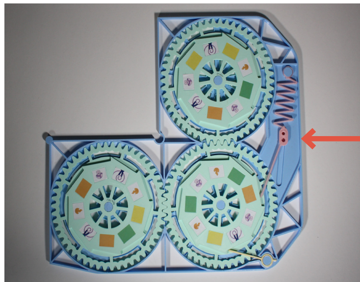
Figure 55: Scroll button mechanism
