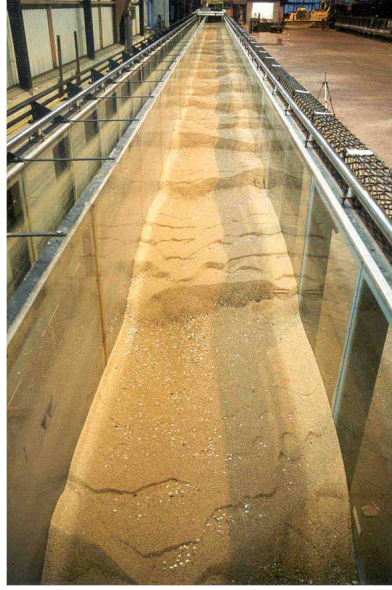
Figure 1.1: Flume experiment for dunes at Delft Hydraulics (Blom et al., 2003)
