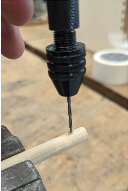
Fig 107: Using hand drill for hole since wood is very soft
