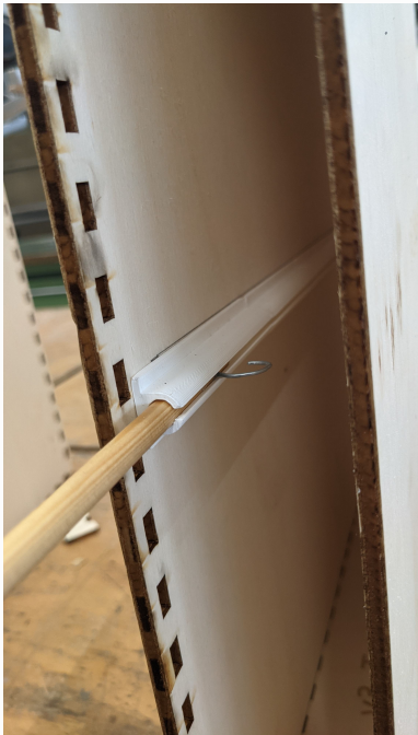
Fig 100: Detail: Pushrod in channel
