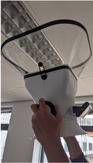
Fig. 47: Device for accurate measurement of exhaust flow rate
