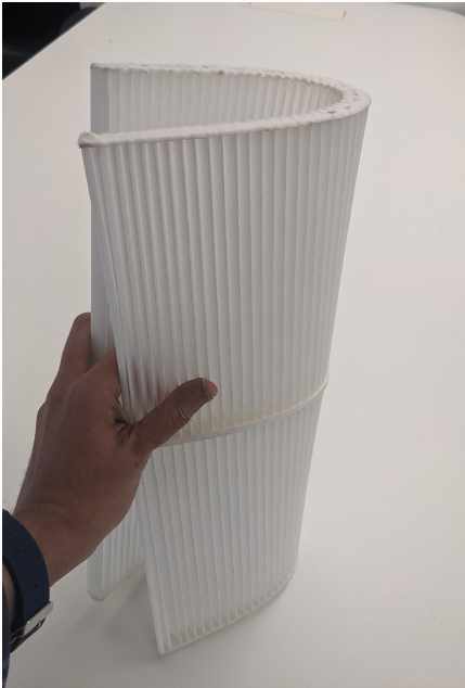
Fig 69: Itho filters deform easily
