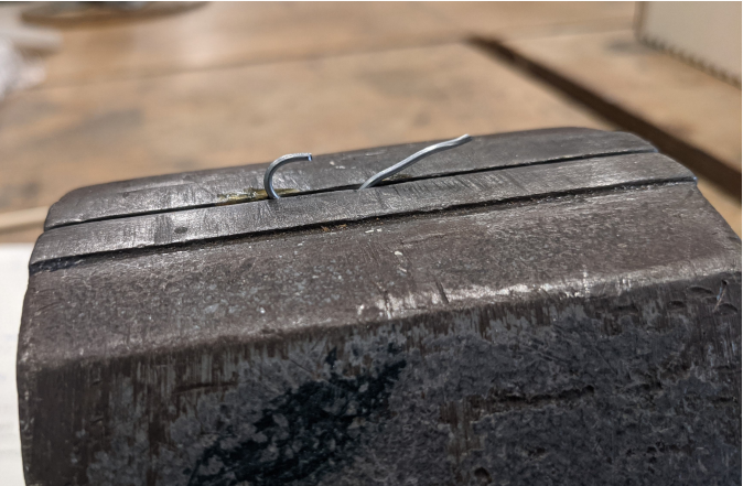
Fig 106: Steel wire bent into hook on vice
