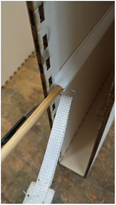
Fig 101: Detail: loop hooked onto pushrod
