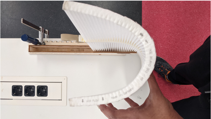
Fig 96: Original Itho filter bending test
