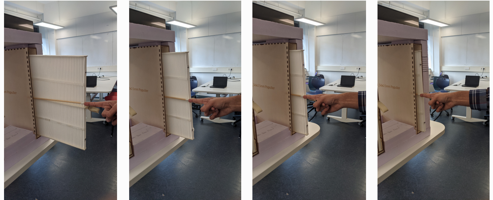
Fig 103: Inserting filter with pushrod
