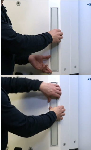
Fig 75: Technician in official user guide first attempts to remove the covers with one hand, then uses both hands applying considerable force.
