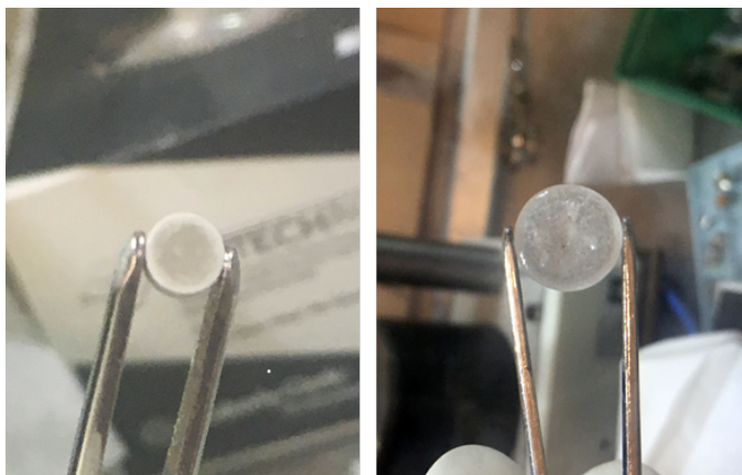
Figure 3.1: Photo of a pressed pellet of LiF, on the left side, and the re-solidified disk of LiF, on the right side.
