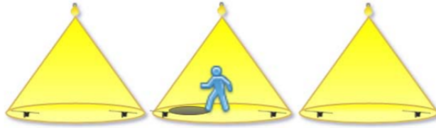
Figure 2.5: Overview of the LocalLight system of E.D. Lascio et al. [4]. Lights on the ceiling and light sensing RFID tags on the floor.
