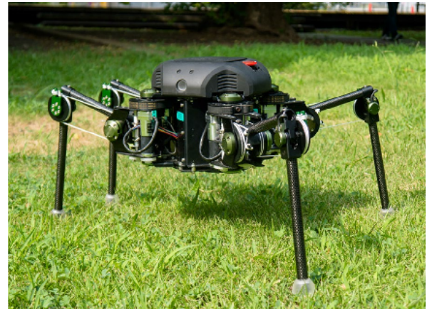
Fig. 9: Quadruped robot TITAN-XIII [16]
