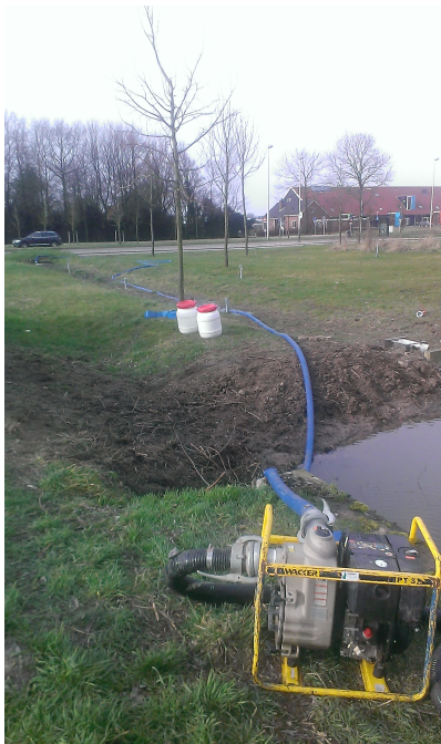
Figure 4.6: Head inflow simulation with a pump
