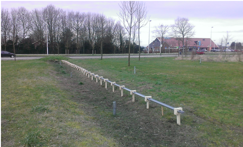
Figure 4.7: Lateral inflow simulation with a gutter system
