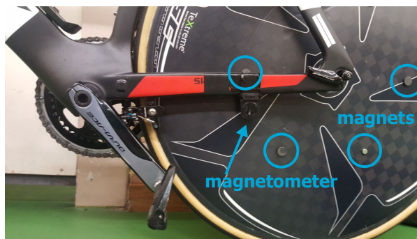
Figure 3.8: Magnetic speed sensor and magnets on the rear wheel
