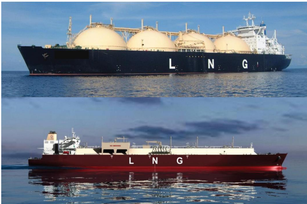
Figure 31: Spherical LNG carrier (upper), Membrane LNG carrier (lower). Source: PIANC (2012)
