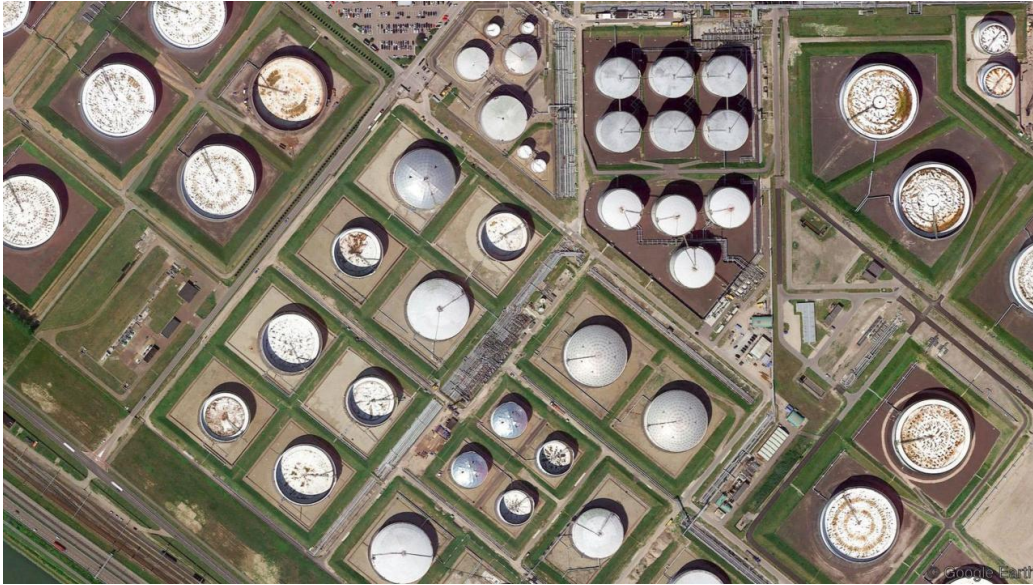
Figure 36: Satellite picture of a liquid bulk terminal with various tank sizes and earth bunds (green squares). Source: Google
