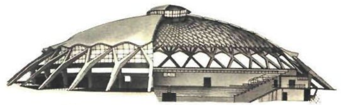
13 The small sport stadium in Rome designed and built by Pier Luigi Nervi in prefabricated reinforced concrete.
