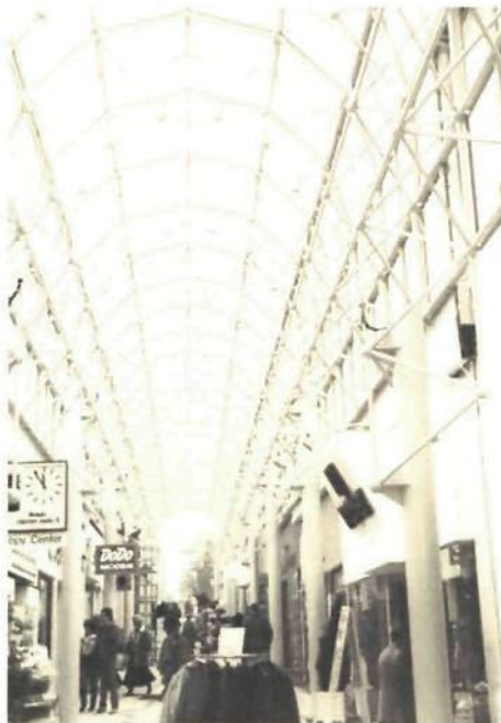
53 Interior of the entrance hall of the insurance company 'Zwolsche Algemeene' in Nieuwegein NL. In plan a diagonally cut square 18 x 18 m surrounded by 2 mirror-glass walls, suggesting visually a space frame 8 times as large as the one really built. Covered with a two-way grid of (intersecting) steel insulated gutters and triple acrylic skydomes on top. As the colours of the gutters are the same as the space frame, visually the beam frame supports the space frame.
