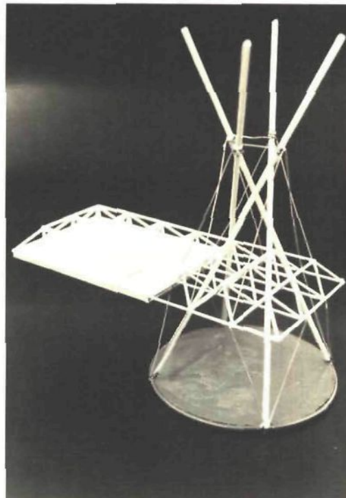
134 Model for an entrance canopy in front of the office of De Nederlanden van 1870 in Diemen (NL): a floating space frame suspended and stabilised by a cable system fixed by 4 tensegrity poles, piercing independently through the space frame. (fig 131) Length of poles 14 m, space frame 5.4x12.6 m. The 4 pole footings rest upon a roundabout in front of the 9 story office building, so that the actual canopy reaches out towards the building. The height of the office tower is balanced by the height of the poles. Designed in 1987 by the author with architect Maarten Grasveld.
