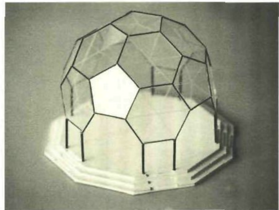
41 Initial design model made by Wiek Röling, consisting of hexagonal and pentagonal faces as a good starting point for further development of the preliminary design.
